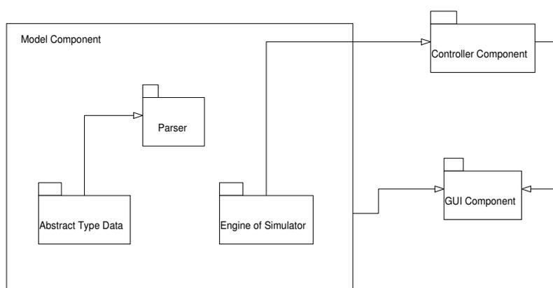
**Fig. 1.** Hierarchical structure and relations among the different components of the application. We underline the package (sets of classes) parser, which contains all functionalities to identify the SBML format and transforms it in an input file of the model. The engine simulator package contains several CLIPS files. The controller package contains libraries to communicate among CLIPS and Java.
