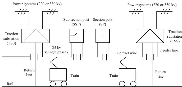
**Fig. 2.** Electrical principle schematic illustration of TPSSs.
