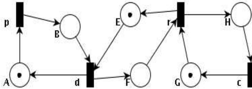
Fig. 3. PTL-net model of a producer/consumer system.
