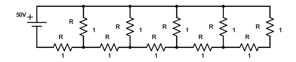
3. Ladder circuit assembly with  $V_0 = 50$  and  $\tau = 1$ . The maximum size is n = 5
